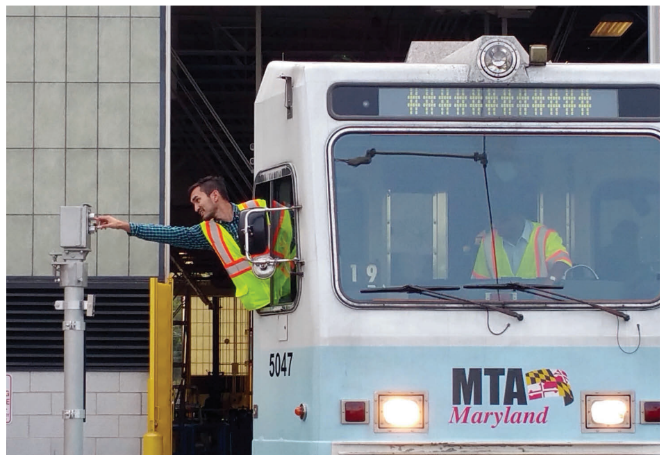
AECOM North Avenue Yard Route Pushbutton System
